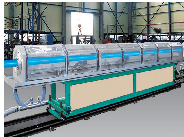
SPRAY COOLING BATH
